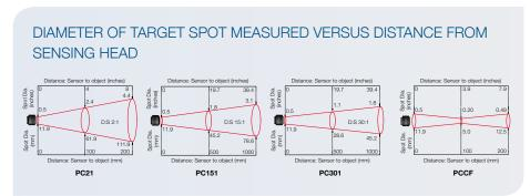
All PyroCouple sensors are fitted with precision Germanium lenses for accurate optics. Model PC21 has 2:1 optics making it suitable for most applications where the sensor can be mounted close to the target. Model PC151 is designed for small or distant targets and has an optical resolution of 15:1. Model PC301 is designed for very small or distant targets and has an optical resolution of 30:1. Model PCCF is designed for targets as small as ø5mm at a distance of 100mm from the sensor.
